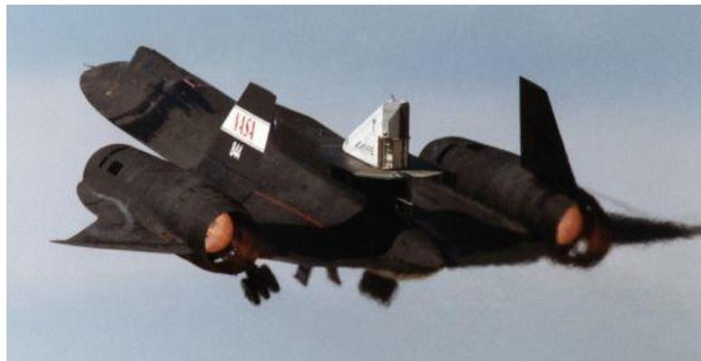
**Figure 1.3: Linear Aerospike SR-71 (BLACK BIRD) Experiment (LASRE)**
